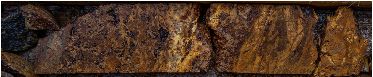
Figure 3: Drill core from hole SR20-29 – Textural example of high-grade gold mineralization present within the Domino zone – sample above graded 19.9 g/t gold and 71.6 g/t silver over 0.94 metres. The host felsic volcanic rocks are cut by an oxidized, vuggy, sheared quartz vein with intense limonite alteration. All primary textures have been destroyed by strain and alteration. Thin bands of chlorite and sericite trend along shear fabric. Shear contains ~15% pyrite and ~5% pyrrhotite. The length of the image is ~30 cm.
